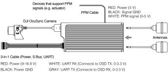
YELLOW: S.Bus (Connects to Flight Controller RX, 0-3.3 V)
