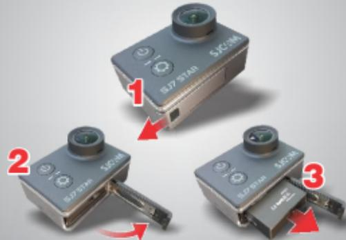
Remove your battery by pressing the button and sliding the lock at the bottom of the camera to release the compartment door.
