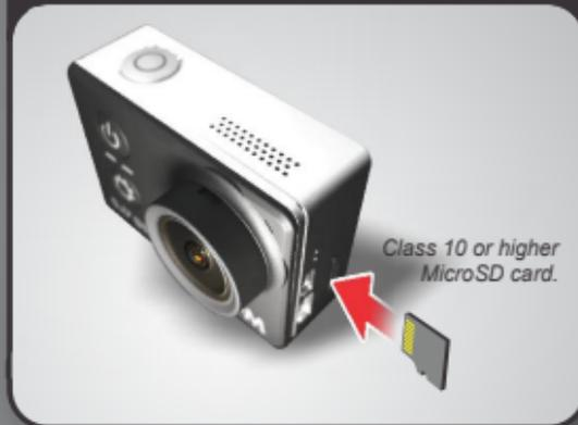
Insert a MicroSD card as shown in the illustration above, with the label facing the touchscreen LCD, until it clicks into place. To remove, just push it in gently and the card will eject.
