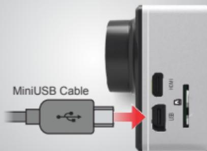
Plug the MiniUSB cable to the slot on the side of the camera as indicated above, and the other end to a USB wall charger with an output of 5V 1A, or plug it to a computer.
