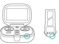
As the controller's battery is used, one battery status light blinks, then turns off. This pattern continues until all lights are off, indicating that the battery is fully drained.
