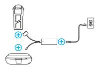
Connect the charger to a wall outlet. The battery status lights on the battery and the controller indicate the charge level.
