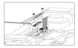
6. Tighten the cover onto the dual downward gimbal connector with screws.
