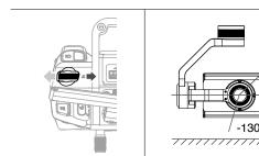
The left dial controls the gimbal tilt. Turn the dial to the right, and the gimbal will shift to point upwards. Turn the dial to the left, and the gimbal will shift to point downwards. The camera will remain in its current position when the dial is static.
