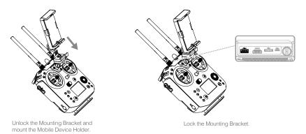
Attach your mobile device, then tighten the clamp to secure it. Connect your mobile device to the remote controller with a USB cable. Plug one end of the cable into your mobile device, and the other end into the USB port on the back of the remote controller.
