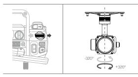
The right dial controls the gimbal pan. Turn the dial to the right, and the gimbal will shift clockwise. Turn the dial to the left, and the gimbal will shift counter clockwise. The camera will remain in its current position when the dial is static.
