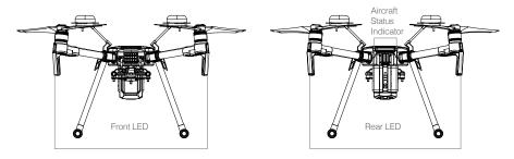
The Front LEDs show the orientation of the aircraft. Front LEDs glow solid red when the aircraft is turned on to indicate the front (or nose) of the aircraft. Front and rear LEDs can be turned off in the DJI GO 4 app. The Aircraft Status Indicators communicate the system status of the flight controller. Refer to the table below for more information about the Aircraft Status Indicators.
