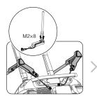
Thread the Datalink Pro antennas through the clips. Make sure that the lines of the antennas lie in the grooves of the mounting board where the clips attach to prevent the antennas from being damaged.
