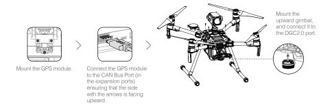
Follow the steps below to mount the Upward Gimbal and GPS Module on the M210 RTK:
