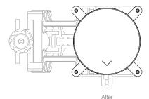
DO NOT try to remove the GPS antenna without first removing the four screws that hold it in place as doing so could damage the antenna.
