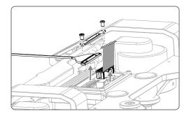
4. Remove the three screws on the top of the single downward gimbal connector.
