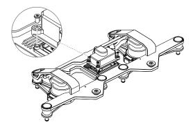
Connect the gimbal signal control cable and gimbal video coaxial cable to the dual downward gimbal connector accordingly. Tighten the spring pad with screws to secure the gimbal video coaxial cable.
