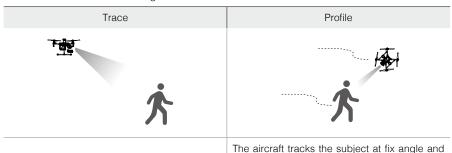
The aircraft tracks the subject at a fix distance. Use the roll stick on the remote controller or the slider in DJI GO 4 to circle the subject.
