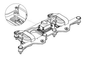
3. Disconnect the gimbal signal control cable and gimbal video cable from the dual downward gimbal connector.
