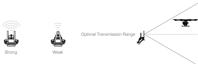
The signal transmission between the aircraft and the remote controller performs best when the aircraft is within the optimal transmission range. Open up the antennas on the remote controller to optimize transmission range. Ideally, the flat surface of the antenna should be facing the aircraft. If the signal is weak, fly the aircraft closer to you.
