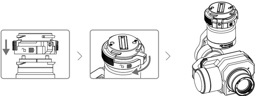
2. Mount the Zenmuse XT onto the aircraft by securing the gimbal adapter.
