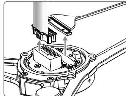
4. Remove the four screws on the top of the dual downward gimbal connector.
