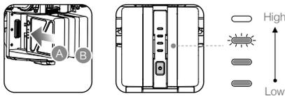
**⚠** Only use battery slot B when using one battery to supply power.
