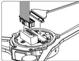
6. Tighten the cover onto the single downward gimbal connector with screws.
