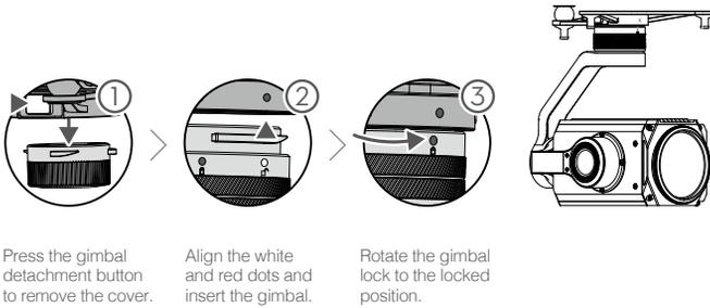
**⚠** Make sure to press down the gimbal detachment button when rotating the gimbal lock to remove the gimbal and camera. The gimbal lock should be fully rotated when removing the gimbal for the next installation.
