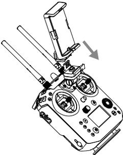
Unlock the Mounting Bracket and mount the Mobile Device Holder.
