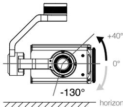
The left dial controls the gimbal tilt. Turn the dial to the right, and the gimbal will shift to point upwards. Turn the dial to the left, and the gimbal will shift to point downwards. The camera will remain in its current position when the dial is static.
