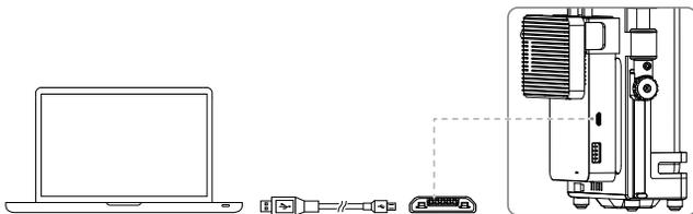
4. Connect the Datalink Pro Ground System to the computer and toggle the 4-position Switch to the COMBO position to activate the Datalink Pro Ground System.
