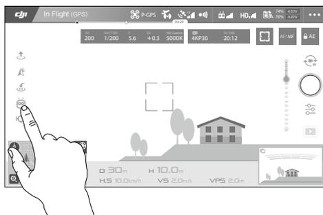
3. Tap once on the target and wait for the “GO” icon to appear. Tap the “GO” icon to confirm the selection and the aircraft will automatically fly toward the target.
