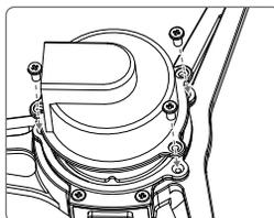
7. Mount the single downward gimbal connector to the aircraft using the three damping balls.
