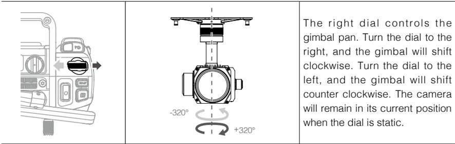
The right dial controls the gimbal pan. Turn the dial to the right, and the gimbal will shift clockwise. Turn the dial to the left, and the gimbal will shift counter clockwise. The camera will remain in its current position when the dial is static.
