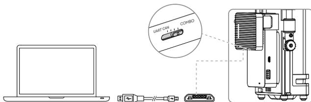
5. Connect the Datalink Pro Air System to the computer and toggle the 4-position Switch to the COMBO position to activate the Datalink Pro Air System.
