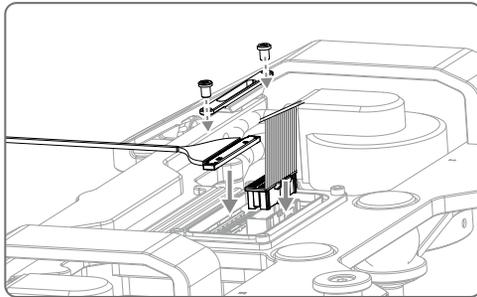
6. Tighten the cover onto the dual downward gimbal connector with screws.
