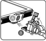
Ensure that Part B is unlocked. Install Part B into Part A.
