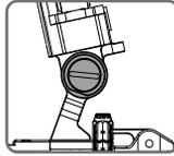
Use a coin to adjust the tightness of the pitch axis.
