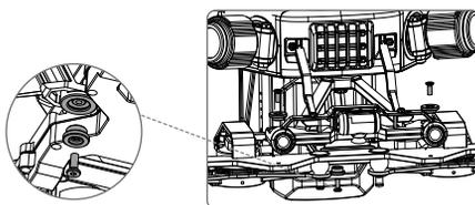
2. Remove the four screws on the top of the dual downward gimbal connector.
