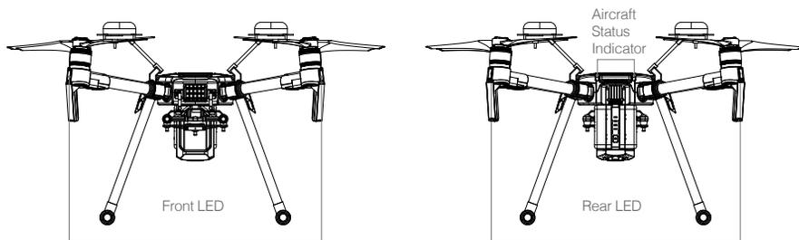
The Front LEDs show the orientation of the aircraft. Front LEDs glow solid red when the aircraft is turned on to indicate the front (or nose) of the aircraft. Front and rear LEDs can be turned off in the DJI GO 4 app. The Aircraft Status Indicators communicate the system status of the flight controller. Refer to the table below for more information about the Aircraft Status Indicators.
