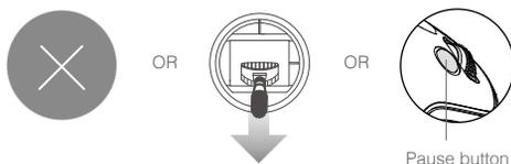
The aircraft will stop and hover after exiting from TapFly. Tap a new target direction to continue flying or begin manual flight.
