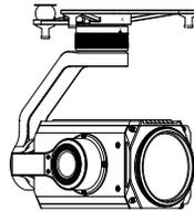
⚠ Make sure to press down the gimbal detachment button when rotating the gimbal lock to remove the gimbal and camera. The gimbal lock should be fully rotated when removing the gimbal for the next installation.
