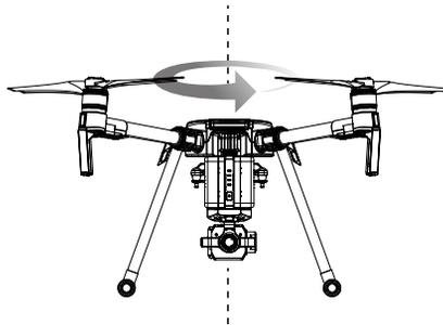
3. Hold the aircraft vertically, with the nose pointing downward, and rotate it 360 degrees around the center axis. Re-calibrate the aircraft if the aircraft status indicators blink red.
