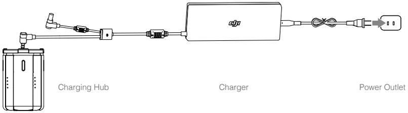
\* It will take approximately 1.5 hours to fully charge the Matrice 200 Intelligent Flight Battery, and 3 hours for the remote controller. It will take a longer time to charge the Intelligent Flight Battery and remote controller together.
