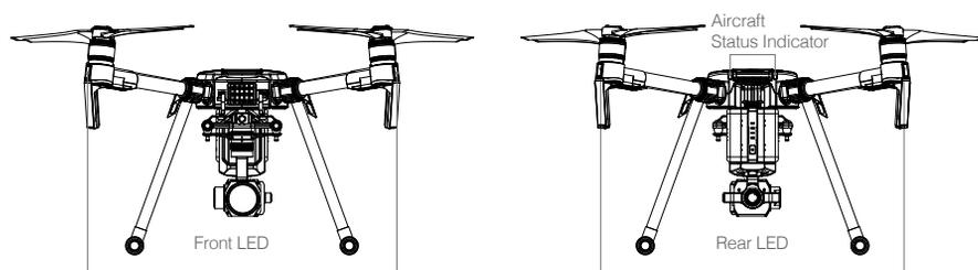
The Front LEDs show the orientation of the aircraft. Front LEDs glow solid red when the aircraft is turned on to indicate the front (or nose) of the aircraft. Front and rear LEDs can be turned off in the DJI GO 4 app. The Aircraft Status Indicators communicate the system status of the flight controller. Refer to the table below for more information about the Aircraft Status Indicators.
