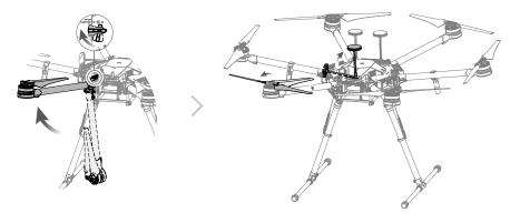
For storage, remove the landing gears, lower the retractable modules, then lower the frame arms to prevent damage.
