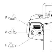
P-mode (Positioning): P-mode works best when GPS signal is strong. There are several states in P-mode which are automatically selected by the Matrice 600 Pro depending on GPS signal strength:
