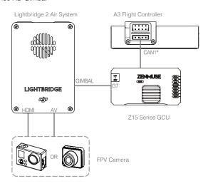
\*You can connect the CAN cable to the CAN Hub on the GPS cable.
