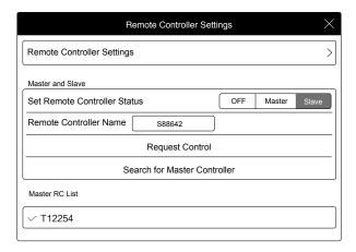
Select the name of the remote controller from the Master RC List and input the connection password to connect to the desired Master remote controller.
