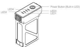
Powering On: Press the Power Button once, then press again and hold for 2 seconds to power on.
