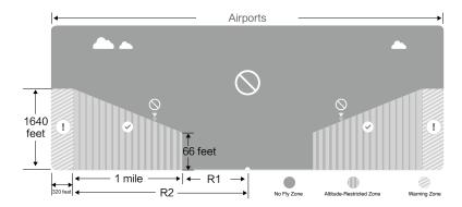
Airport No Fly Zones are comprised of a no fly zone and an altitude-restricted zone. Each type of zone encompasses a radius of a certain size.
