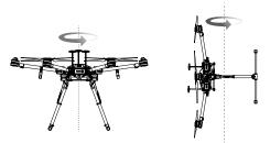
4. Recalibrate the compass if the Aircraft Status Indicator blinks red.
