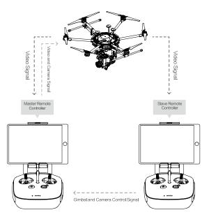
Use the gimbal dial on the remote controller to tilt the camera in the Single Remote Controller mode. In Dual Remote Controllers mode, use the Slave remote controller to tilt, pan or roll the camera.
